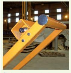
Safety light beams fitted to press carriage.
